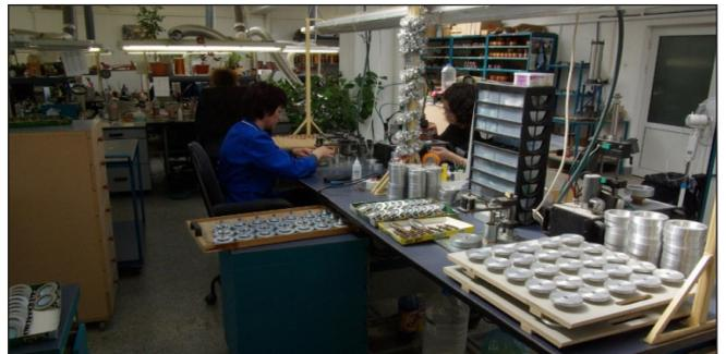
Photo 3: Oberton's compression driver assembly work station
