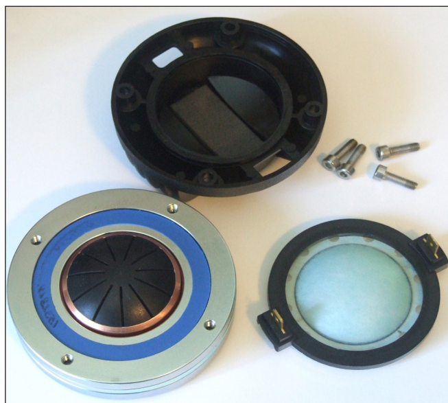
Photo 2: The ND45 has a 44 mm (1.75") diameter two-layer voice coil wound with aluminum wire wound onto a Kapton former driving a polyester sandwich diaphragm and vented surround.
